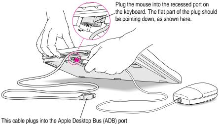
This cable plugs into the Apple Desktop Bus (ADB) port on the back of the computer. The ADB port on the computer is marked with the  $\mathbb{P}$  icon.
